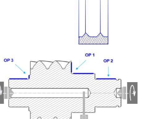
Grinding technology Kiss Grinding
