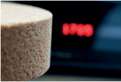
Good vibrations: the e-module checks the density and hardness of the wheel.
