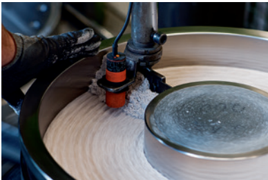
Evenly does it: how the mould is filled determines how round the wheel will be.
